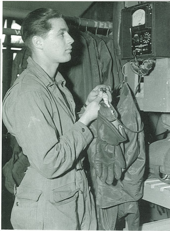
Routine testing of flight equipment ensured against breakdown of vital equipment when operating at high altitude and below freezing temperatures. Here a pair of electrically heated gloves are being checked out on a resistance tester. (Daniels & Kueppers)
